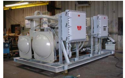
Trane Model RTHD Water-Cooled Chiller AFTER
