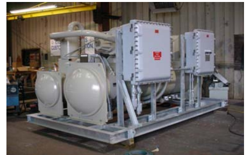
Trane Model RTDH Water-Cooled Chiller AFTER
